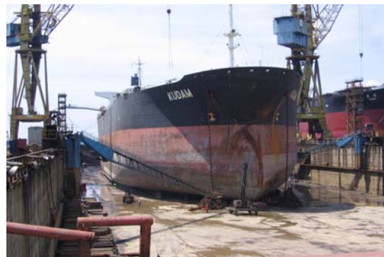
The 'Kudam' oil tanker in dry dock in the Philippines undergoing conversion works
